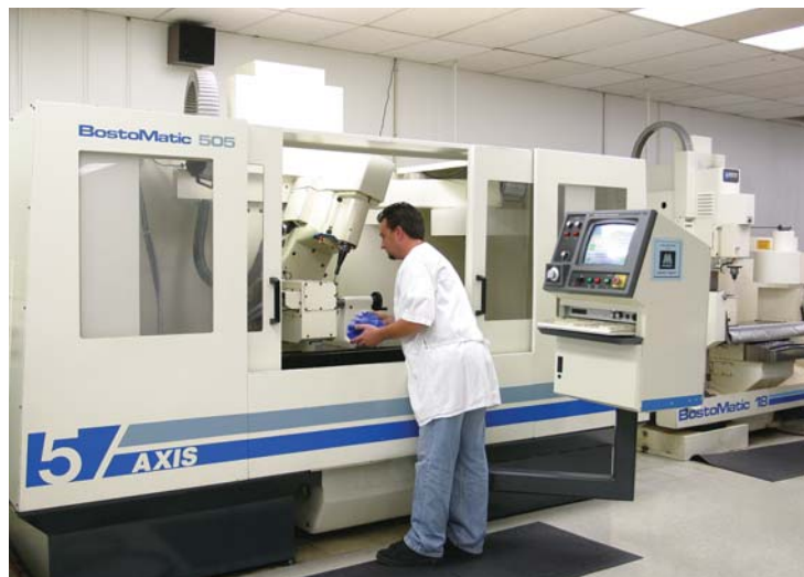
Kevin Miller, CNC mill operator, sets up to machine a turbine mill on a Bostomatic 505 5-axis CNC mill.
