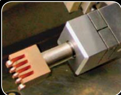
A rotary table can be used as an indexer to rotate the work piece into position before cutting starts.
