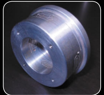
Rotary axis movement makes it possible to cut small, complicated slots. Slots with tapered walls are also possible.
