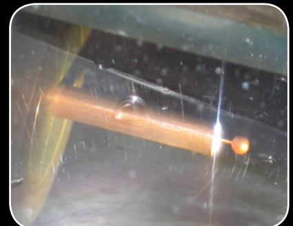
A high-speed spindle can rotate continuously at speeds up to 1500 RPM for EDM turning operations.
